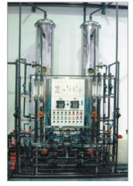
Compared with the reverse osmosis device introduced in recent years, it has the advantages of completely removing ionic impurities; Low requirements for water pretreatment; The
